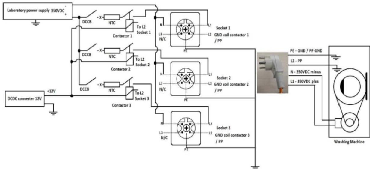
**Figure 5:** DC electrical setup of DC test benches
