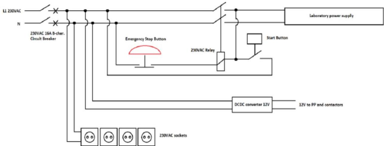
Figure 1: AC electrical setup of DC test benches
