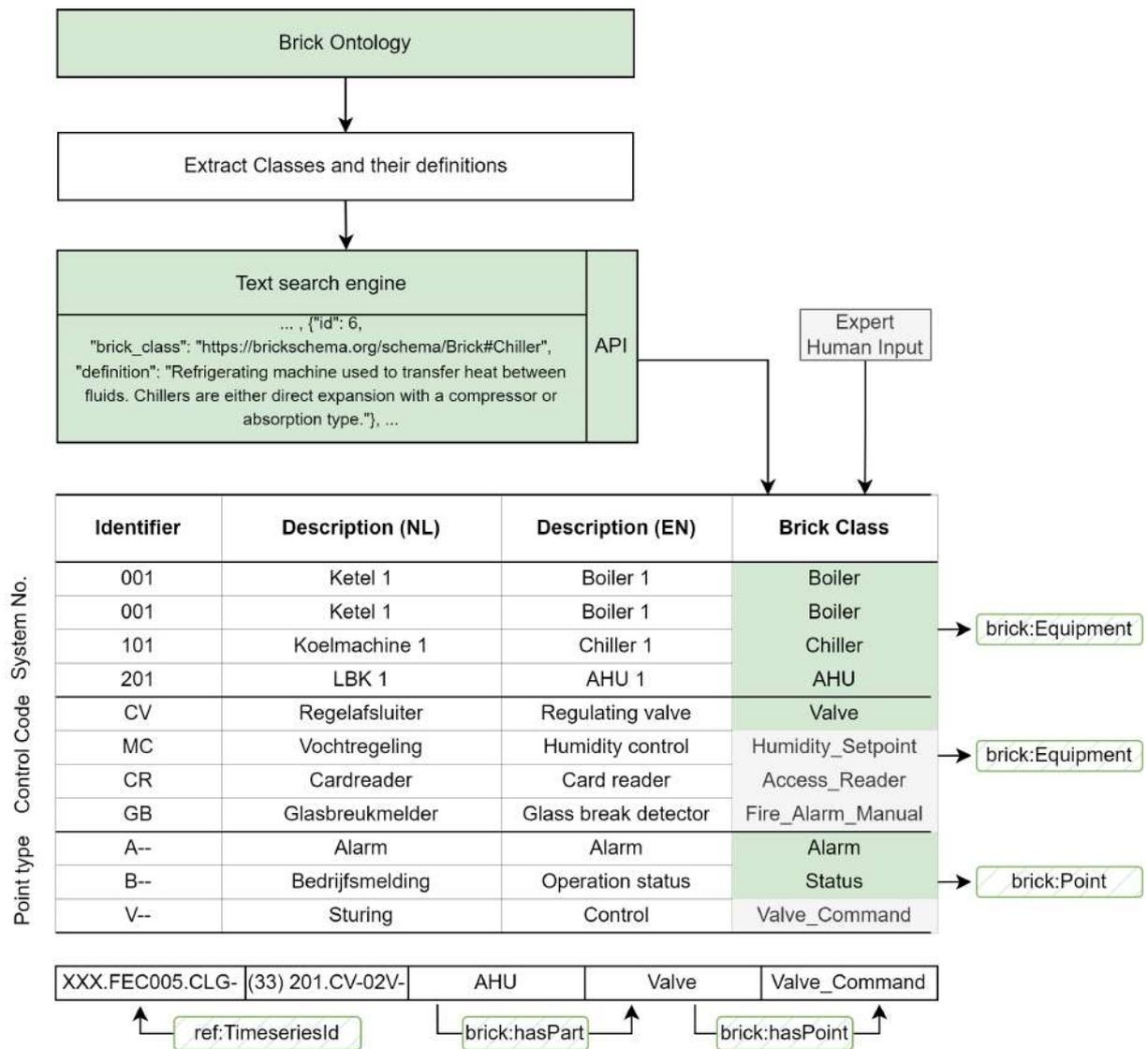
Figure 2 Workflow of mapping to Brick Ontology
