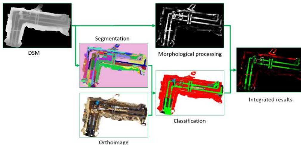
Figure 2. The procedure of the proposed method to detect utility items combining the classification and morphological processing.
