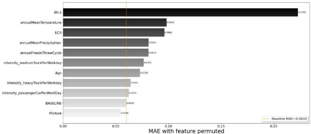
Figure 3: The permutation feature importance of the GRU model for the regression of IRI
