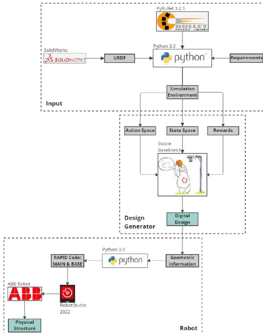
Figure 1: Design and construction process for dry-stacked structures
