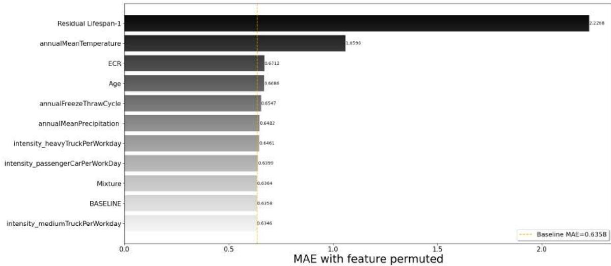
Figure 2: The permutation feature importance of the RF model for the regression of residual lifespan
