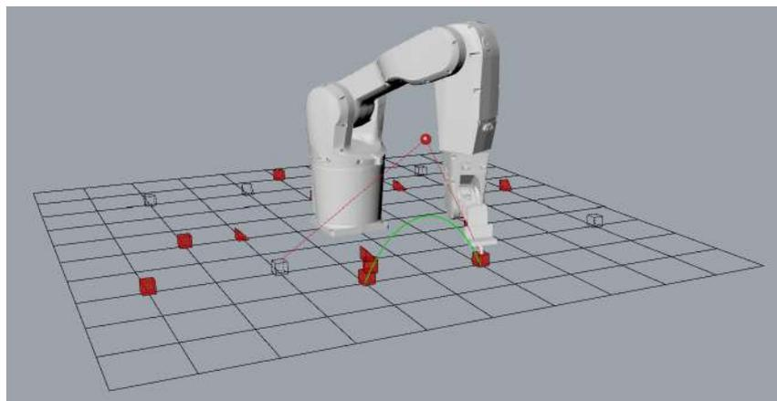
Figure 2: Path-planning for robotic construction
