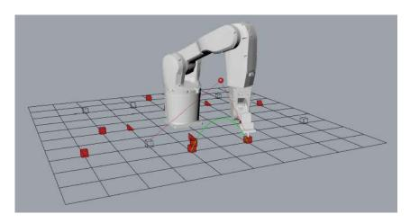
Figure 2: Path-planning for robotic construction
